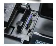
Secure SD Port SD Card Utilities include program save/load, report capture, firmware updates plus graphics up and downloading. The SD port, hidden under the printer cover, is secure from tampering.
