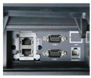
Secure Connector Panel Up to four RS-232C communication ports hidden behind a convenient, easy to access door located on the back of the unit.
